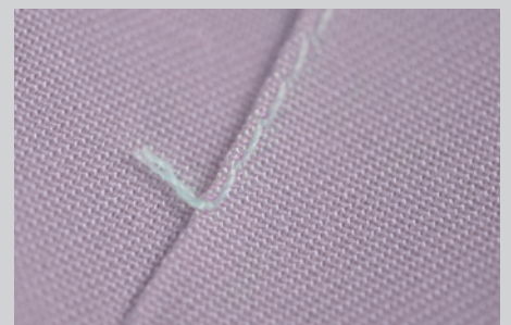
Clean-cut at end of the seam (< 5mm)
