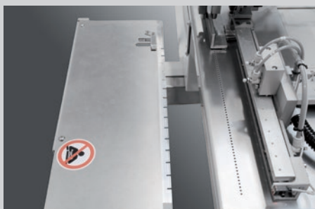
Larger feed table for double-pointed darts (Option on -23/11, -23/12)
