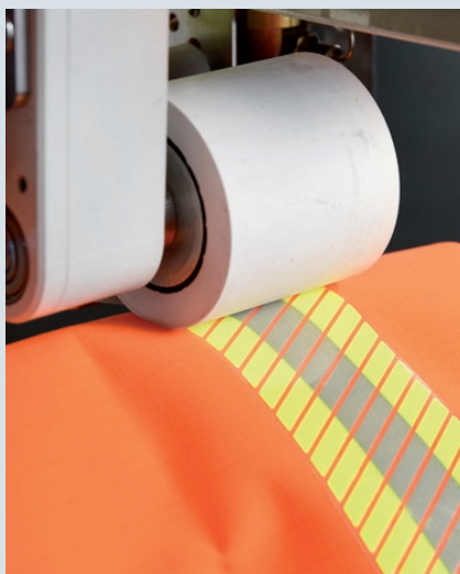
焊接贴合反光条 Welding of reflective strips
