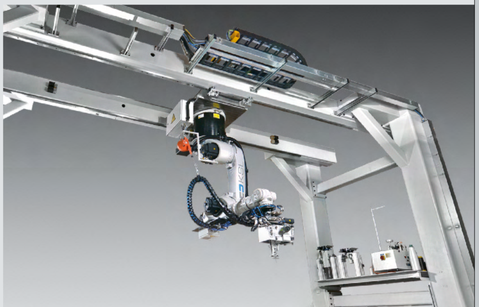
3D-Roboter in Portal-Bauweise 3D robot system with portal Robot 3D tipo pórtico
